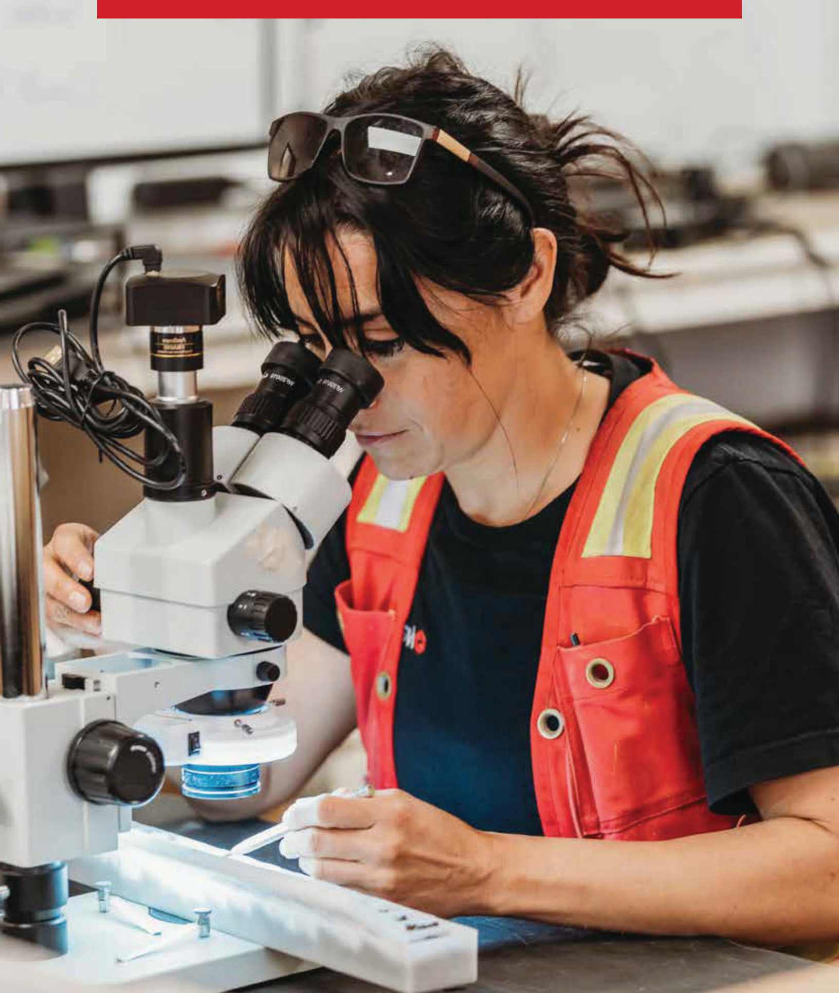
Sarah Bala, Geologist, logging drill chips produced by reverse circulation exploration drilling at Santa Cruz Copper Project
